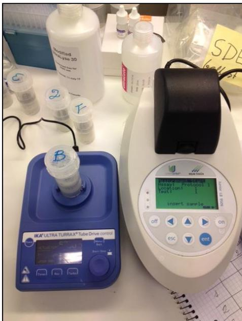
**Figure 1** Picture of the luminometer (on right) for ATP measurement developed by Aquatools with the grinding device (on left) to mix the sample in the grinding tube containing beads for ATP extraction.
