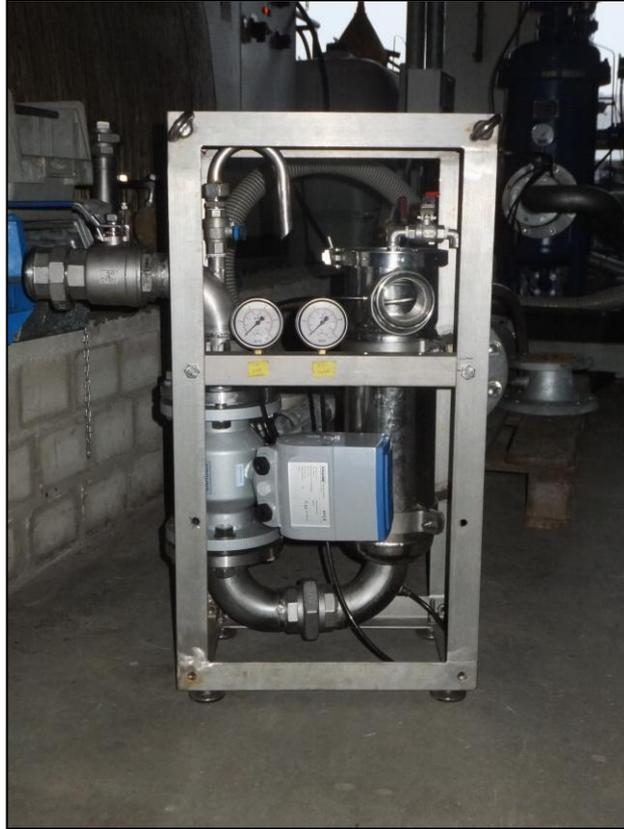
Figure 3 : Ballast water sampling system Prototype 01
