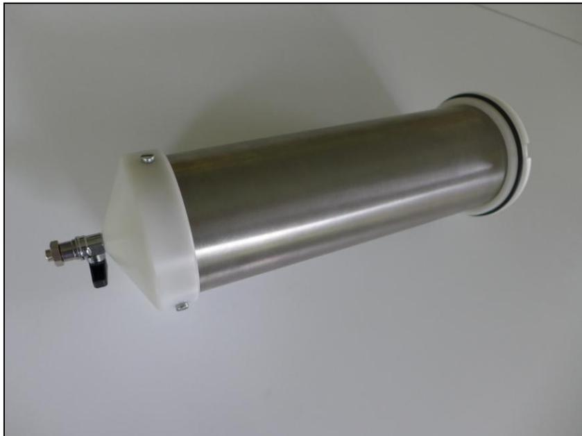
Figure 4 : Filter screen 50µm of the ballast water sampling system 'Prototype 01'
