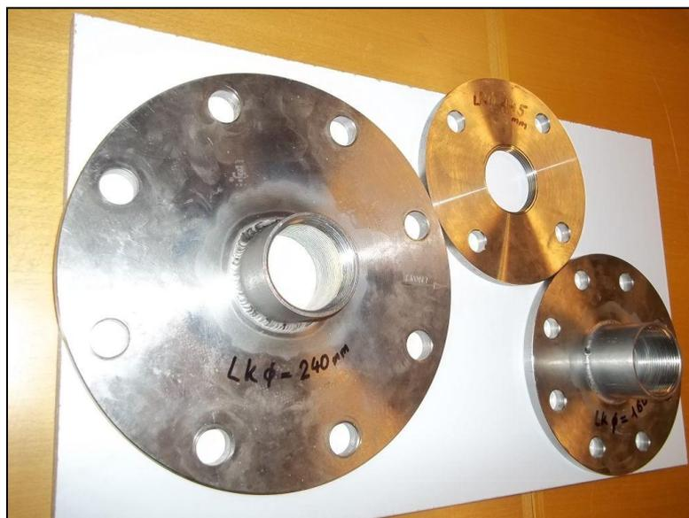
Figure 8 : Flanges of different size for application with the universal sampling port
