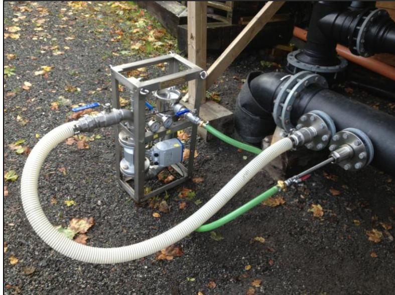
Figure 10 : The sampling system connected to a ballast water pipe system with : universal sampling port (flange on the right, green tube, the sampling system 'Prototype 01' and the back flush port (flange on the left, white tube)
