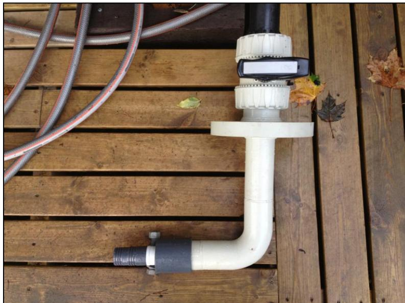
Figure 6 : "L" shaped isokinetic sampling port disconnected from main ballast water pipe
