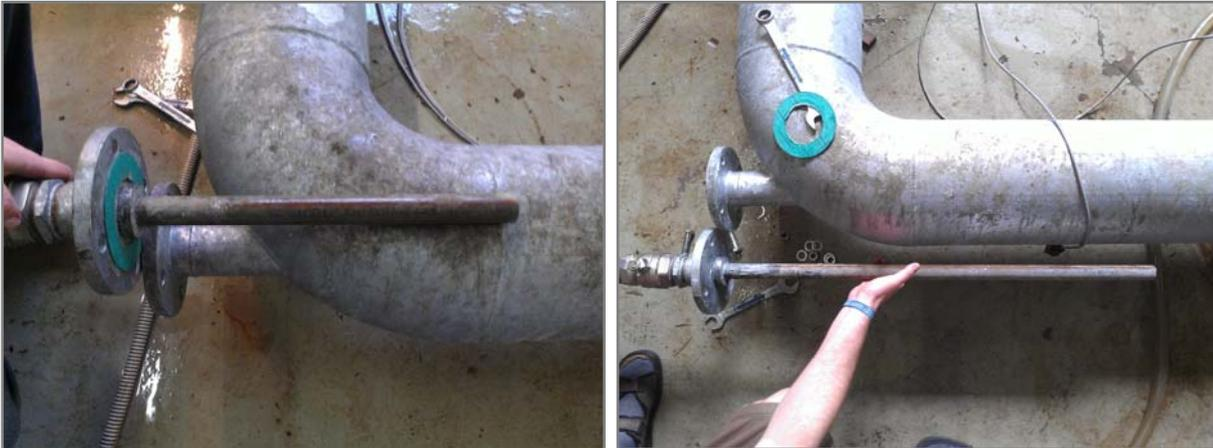
Figure 5 : Isokinetic sampling port “bend” type : definition of “length”, left: 0 cm, right: 50 c
